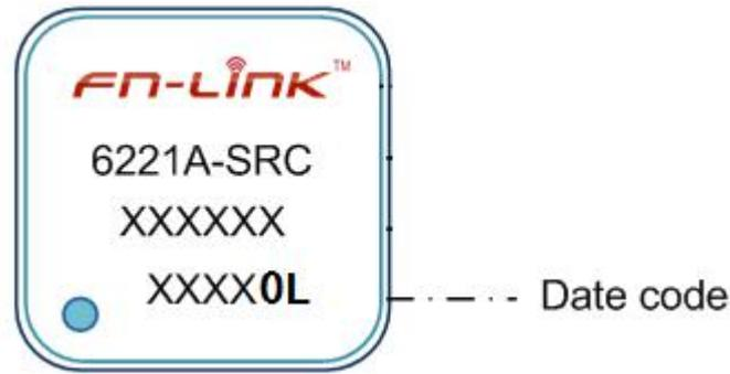
NOTE: datacode '0L' is P/N: FG6221ASRC-0L
