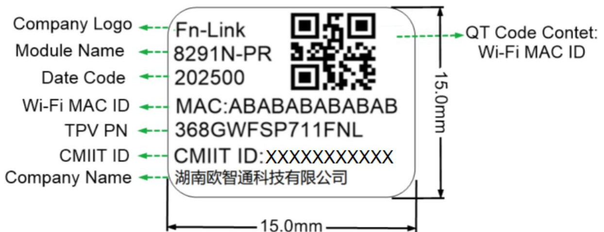
Figure 5-1 Label Marking description
